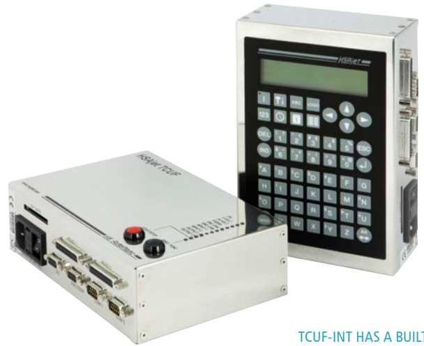
TCUF-INT HAS A BUILT-IN KEYBOARD AND DISPLAY
