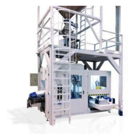
AUTOMATIC BAGGING MACHINE FOR THERMO-SEALED BAGS WITH INTEGRATED WELDING SYSTEM
